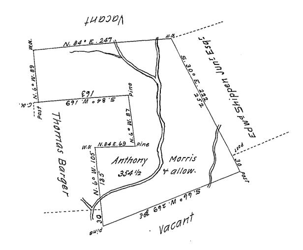
A draught of a tract of land called \_\_\_\_\_\_ situate on both sides of the path leading from Ellis Hughes at Catawassey to obliterated adjoining and between land surveyed for Thomas Barger and Edward Shippen Jun! Esg! in the County of Northumberland containing three hundred and fifty four acres and a half besides the usual allowance of 6 ff cent for roads Yta. Surveyed the 9th day of June 1774 for Anthony Morris in pursuance of a warrant dated the 12 day of January 1774.
